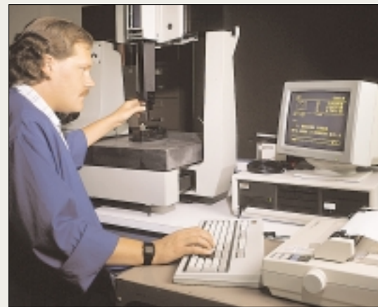
Reynolds Industries Quality Assurance System conforms to the requirements of ISO 9001 Standards. Shown is our Coordinate Measurement Machine for use where full contact measurement is required.
