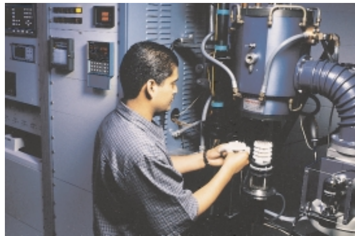
Vacuum furnace with on line mass spectrometer, cryogenic filter and turbo-molecular pump for production brazing of high voltage, high current vacuum trigger switches and other high vacuum devices requiring a ceramic to metal seal.
