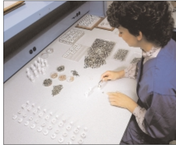
Ceramic fixtures are used to assure precision alignment of metal details during the furnace brazing process.
