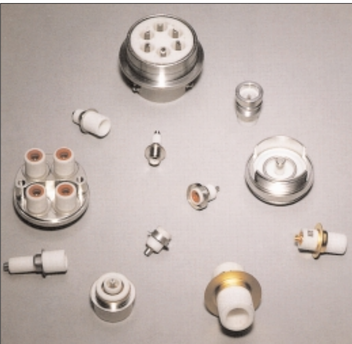
A variety of ceramic-to-metal sealed high voltage connectors. Silicone rubber dielectric seals are added for operation at altitudes up to 70,000 feet. Engineers choose these connectors for long term hermeticity, higher operating temperatures and resistance to radiation.
