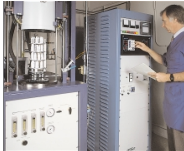
Precision computer controlled temperature/time profiles within the hydrogen brazing furnace, are necessary to the manufacture of repeatable high strength and leak tight ceramic-to-metal connectors and assemblies.
