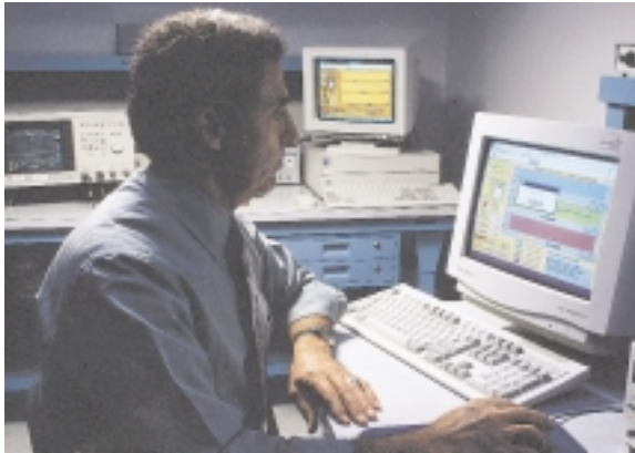
High voltage trigger switches require extensive non-destructive testing on a 100% basis. Shown is a test being conducted to record the trigger voltage level after exposure to cold temperature. The tester is computer controlled and the test data is recorded as a printout and electronic data base.
