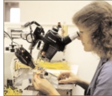
Precision gold bridgewire welding to EBW header electrodes is critical to performance and high EBW system reliability.
