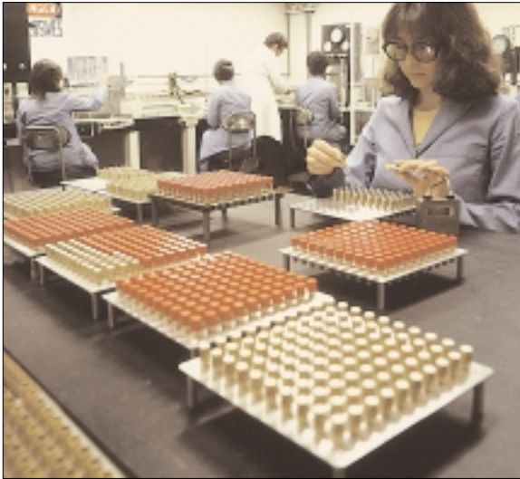
Explosive loading is conducted in a "white-room" equipped with special weighing, loading and lot control equipment needed for "secondary" explosive initiator manufacturing.
