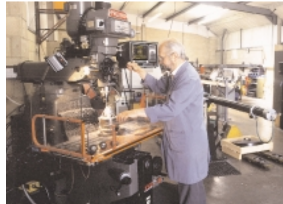
Computer controlled milling, turning and drilling department produces many of our tight tolerance metal and plastic detail parts.
