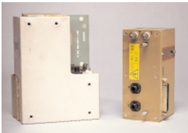
7 KVDC power supply for an airborne radar application. This power supply was designed by the customer and assembled and tested by personnel in the Electronic Products Division using special encapsulation techniques developed at Reynolds Industries Limited.
