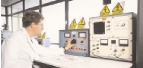
A partial discharge (corona) test being performed.
